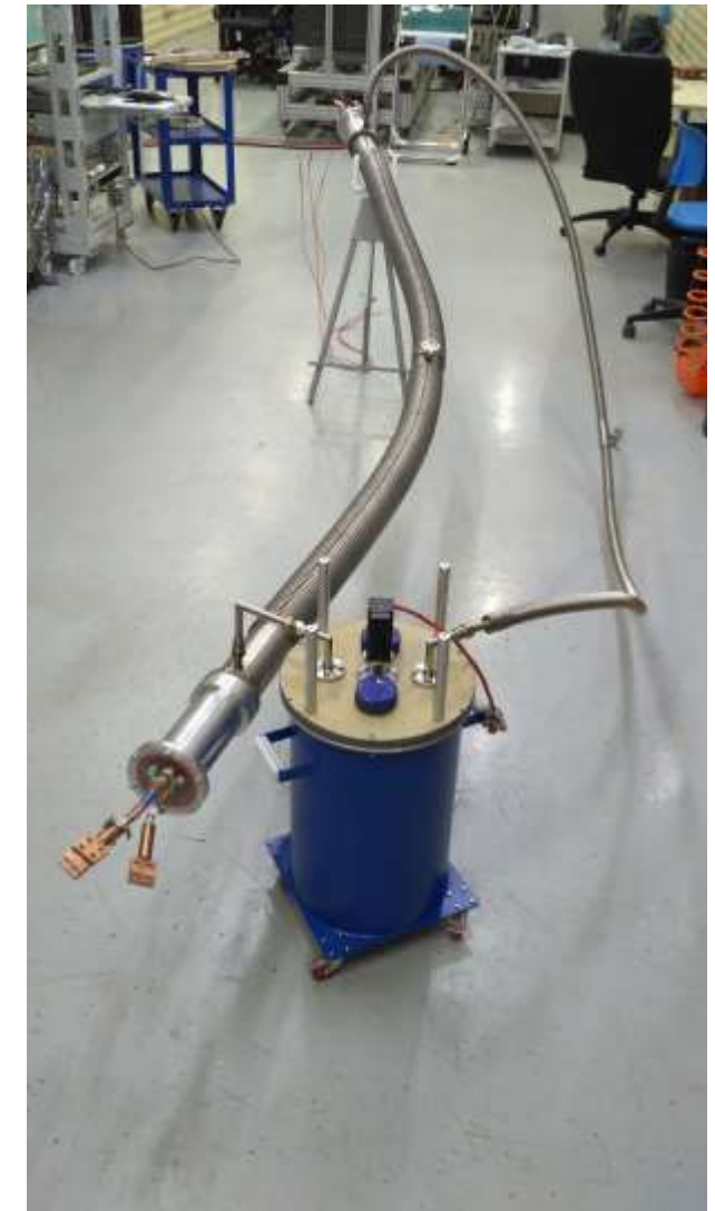
Assembled cable system. Successful acceptance tests in May 2018.
